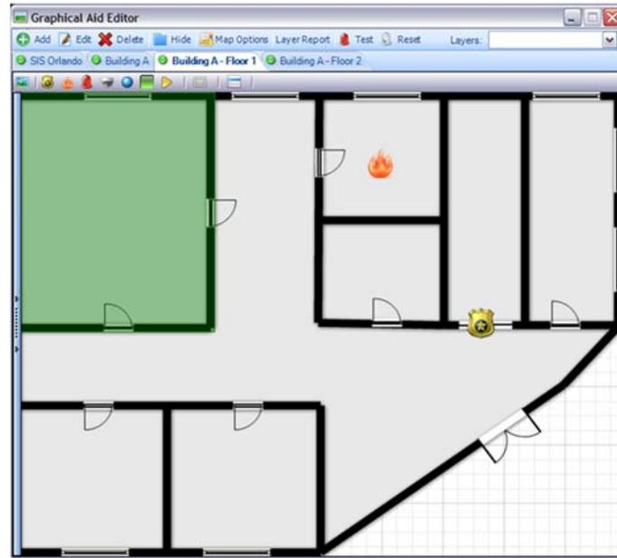
The Alarm Center® Graphical Aid Module “GAM” is used to graphically represent a location’s blueprint by allowing users to diagram their location with images, specify zones locations, and receive zone alarm alerts with animated images.
